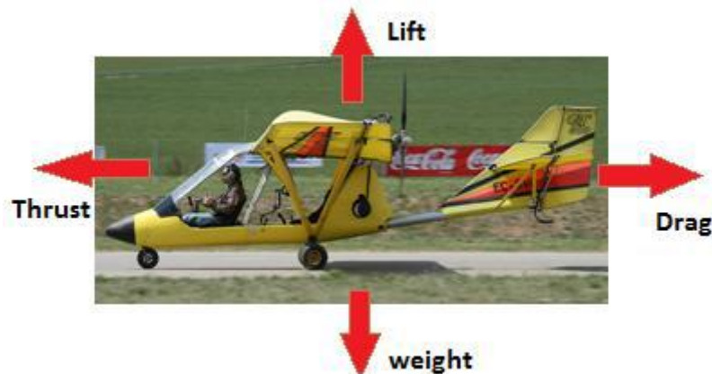
Figure 2.1: Types of load acting on aircraft.
