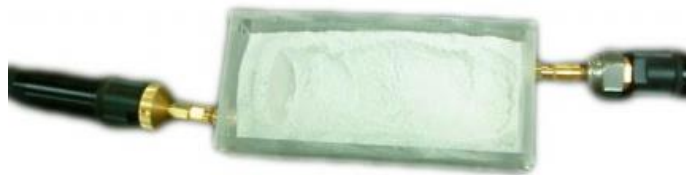
Figure 3: Filter Sensor with the Sample of Rice
