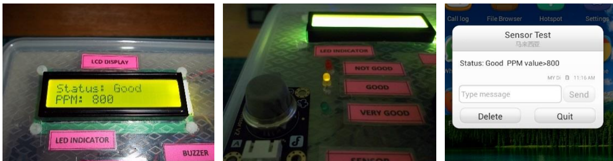
Figure A.2: The Result for "Good" Condition CO 2 Concentration Level Testing
