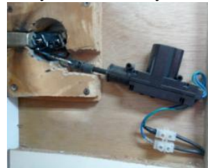
Figure 13: 12V actuator mounted inside the door
