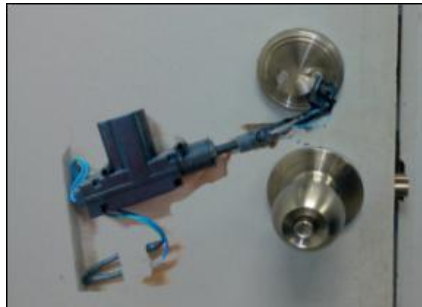
Figure 4: Door lock using actuator.
