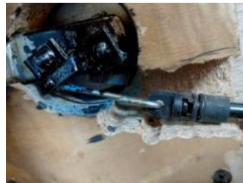
Figure 10: Actuator connects to door knob
