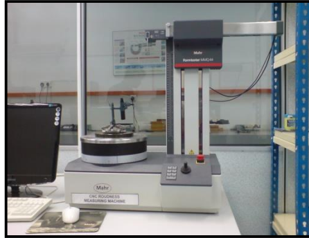
Figure 2.3: The CNC Roundness ó Formtester MMQ44 manufactured by Mahr at the Metrology Laboratory
