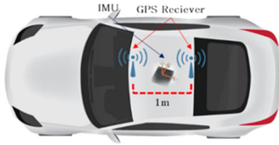
Fig. 4. The setup of environment in vehicle test.
